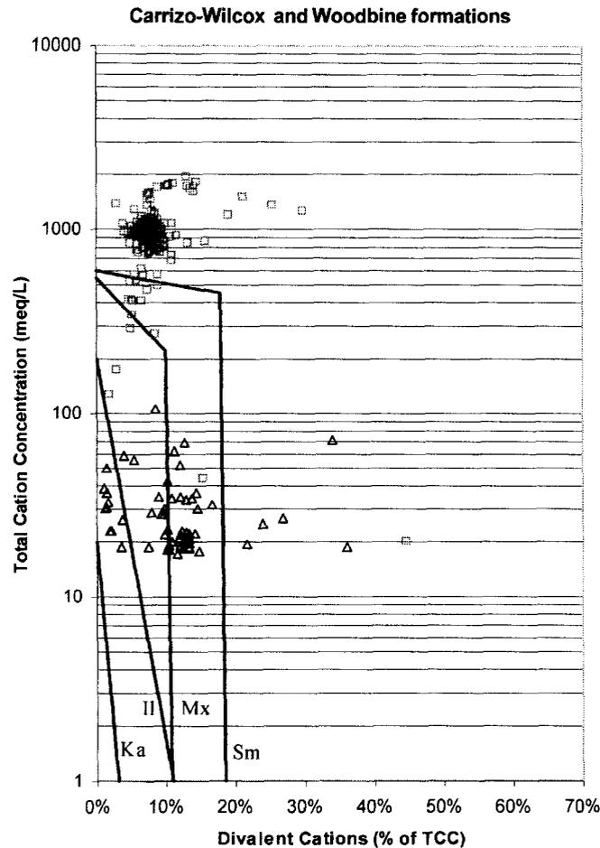
Fig. 5b. Plot of total cation concentration and divalent cations percent for concentrate and formation water (East Texas Basin). Ka = kaolinite; Il = illite; Mx = mixed layers; Sm = smectite; TCC = total cation concentration. Note: any water inside the delineated domain will deflocculate the corresponding clay.
