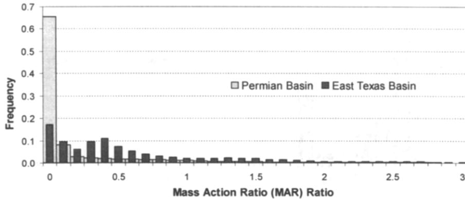
Fig. 6. Computed MAR ratio distributions for the Permian Basin (concentrates from Ogallala and Dockum waters injected into the San Andres formation) and East Texas Basin (concentrates from Carrizo-Wilcox waters injected into the Woodbine formation) (Number of bins: 31; bin size: 0.1; number of trials: 100,000).
