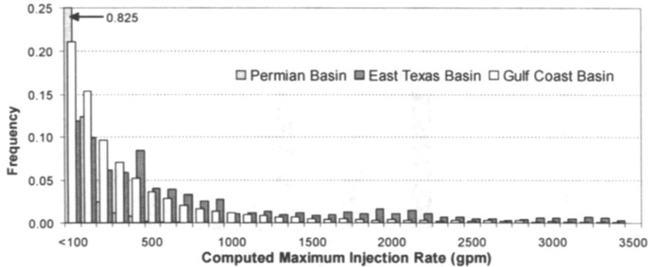
Fig. 9. Distribution of computed maximum injection rates for selected basins (Number of bins: 36; bin size: 100 gpm; number of trials for each basin: 10,000). Note that most of the rates computed for the Permian Basin are less than 100 gpm (100 gpm = 0.0063 m<sup>3</sup>/s).
