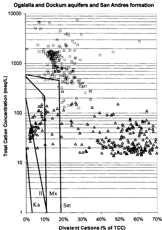
Fig. 5a. Plot of total cation concentration and divalent cations percent for concentrate and formation water (Permian Basin). Ka = kaolinite; Il = illite; Mx=mixed layers; Sm=smectite; TCC = total cation concentration. Note: any water inside the delineated domain will deflocculate the corresponding clay.
