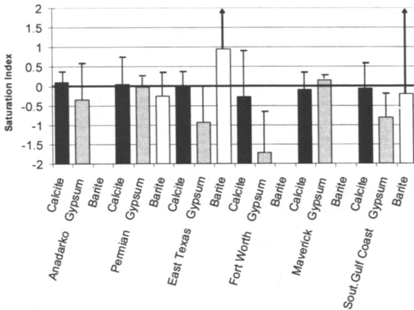
Fig. 4. Summary of computed median values and 95th percentile of saturation index (mixture of formation water and concentrate in different proportions). Arrows indicate saturation index values larger than 2 which is retained as the value beyond which recurrent scaling problems could occur during the injection. Basin locations are displayed in Fig. 1.
