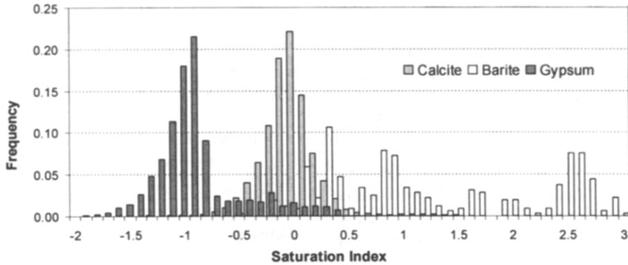
Fig. 3. Selected histograms of computed saturation index of scale forming minerals for mixing of acidified concentrate and formation water in the East Texas Basin (Number of bins: 51; bin size: 0.1; number of data points for calcite: 19,580; gypsum: 19,349; barite: 320).
